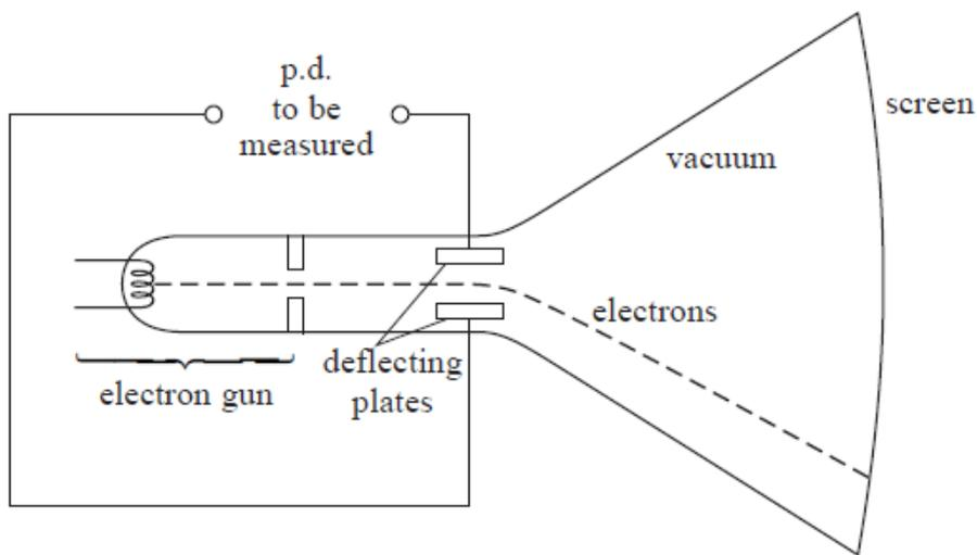
(a) The electron gun includes a filament. When this filament is heated, electrons are released and are accelerated by a p.d. of 1.5 kV to form an electron beam.
