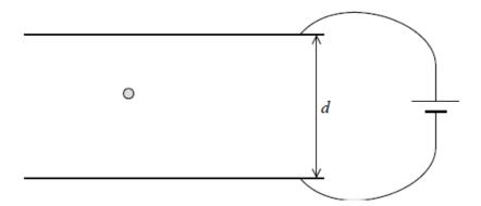
When the p.d. is 0 V the oil drop accelerates to terminal velocity. The p.d. is increased. It is observed that at a particular p.d. V the oil drop stops falling and remains stationary between the plates.
